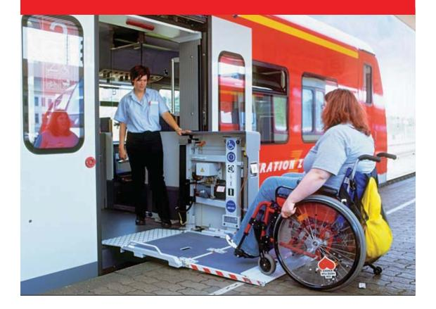
The range of semi-automatic trainlifts provides safe and easy access for wheelchair users travelling by rail. Stowed neatly inside the entrance to the carriage, the platform pivots round and lowers, bridging the gap between the carriage floor and the platform. For reasons of safety the lift is stowed locked and can only be operated by authorised personnel. The Trainlift is designed for lifting up to 1200 mm.
