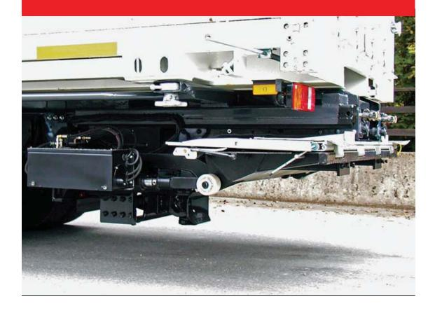
Robust retractable lift available in two capacities specially designed for drawbar applications. Stowing 'completely' out of the way under the rear of the vehicle it is ideal for fork lift and dock loading operations. Suitable for dry freight and refrigerated applications.
