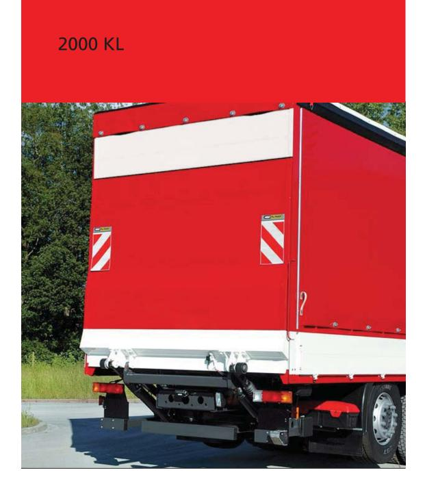
2000 KL is a powerful tail lift for demanding applications that require a lifting capacity of 2000 kg with a load clearance of 750 mm. 5 different lift arms and models with aluminium or steel platforms are available. A wide range of options are available, to meet the requirements of virtually all applications.
