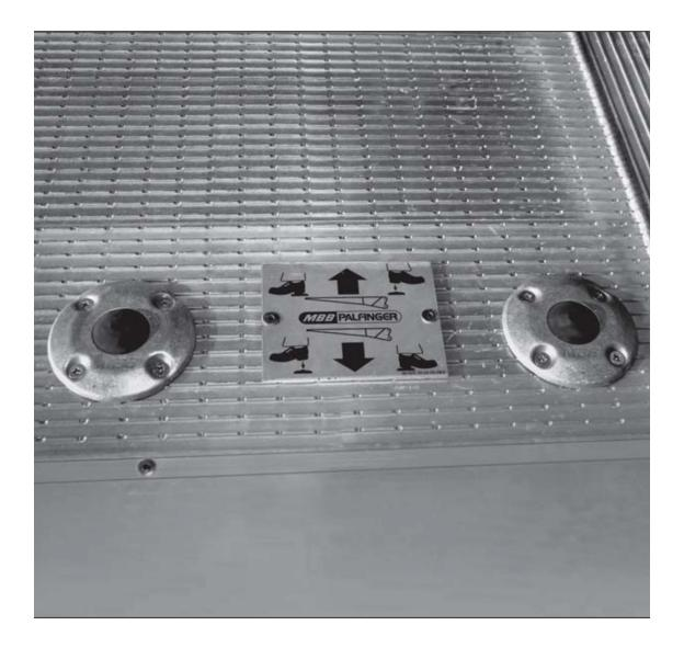
Our 'Intelligent' foot controls are able to distinguish between contact with the operator's foot and the load! Should goods be resting on the foot controls the lift remains static.
