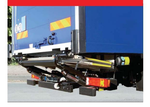
The TwinFold is a light weight, 2-cylinder tuckunder lift with a lifting capacity of 1500 kg. Its folding platform stows under the vehicle chassis, providing clear access to the rear of the vehicle when required. Platforms available 1200 mm and 1400 mm deep. Designed for dry freight applications, it is ideal for the lifting of pallets and roll cages. With its two lift cylinders and two parallel struts, the TwinFold lift offers full stability. Mechanical auto-tilt at ground level.
