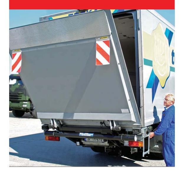
This special lift is designed for fitting to vehicles with a deep coupling system. It uses well-proven standard components of 1500 K and 2000 K lifts. The single-piece underrun bumper is spring-loaded and, on request, hydraulically pivoting. The long lift arm (1100 mm) permits level mounting of the platform.
