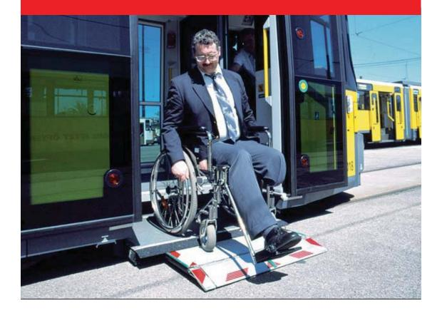
The MEDILIFT range of fully automatic, electrically operated lifts is designed for low-floor trams and buses, providing safe and easy access for wheelchair users. The Medilift is particular useful in areas with no pavements as all passengers, not only wheelchair users, can enter the vehicle with ease.
