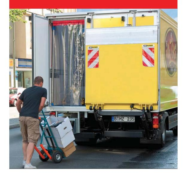
These tail lifts are based on the well-proven K series. They offer a wide range of applications and are tailored to the transportation of fresh or chilled goods. The rear of the truck may be accessed without lowering the 1/3 or 2/3 width platform which may be mounted to the left (K1TL) or right (K1TR) side of the vehicle. Platform widths from 800 mm to 1960 mm.
