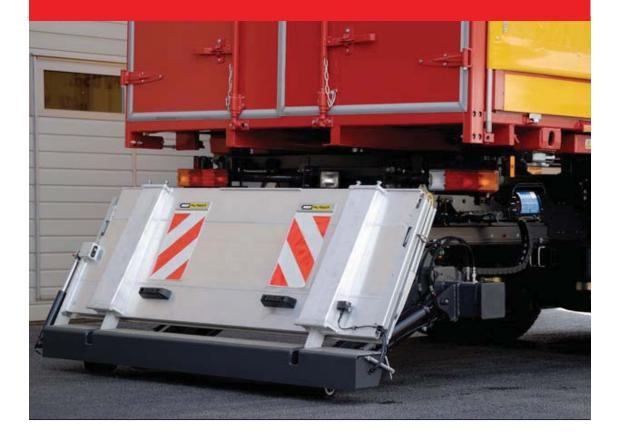
Robust retractable lift with double folded platform ideal for vehicles with demountable bodies and also fixed bodies with short overhangs. The lift including the retraction unit leaves the factory fully assembled with the lift unit powder coated. When stowed, the lift forms the vehicle's underrun bumper. The lift is entirely operated by a user friendly K-plus control system and optional EasyMove control. Ideal for frequent use.
