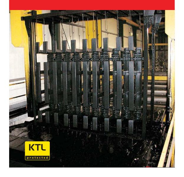
Our lifting mechanisms are also protected with KTL layer as standard. This minimises the consequences of stone chip damage and prevents spreading rust. The KTL coating has been subjected to a Salt-spray test:
