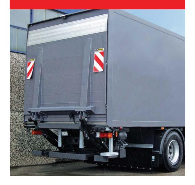
Lifting a full 2000 kg, the 2000 K offers a choice of steel or aluminium platforms, up to a maximum depth of 2800 mm and is frequently chosen for use by the food and drink distribution industry. The 4-cylinder lift mechanism is available with four different lift arms, ranging from 700 mm to 1100 mm.
