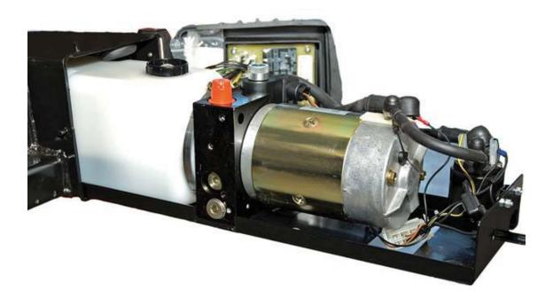
The power pack is housed in the main beam, out of harms way, and is easily pulled out for inspection and maintenance. In addition, noise from the hydraulic pump is greatly reduced when the lift is being used in residential areas or at night.
