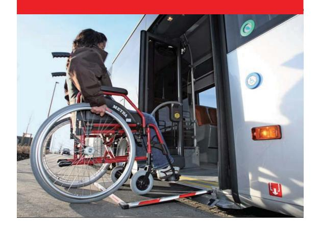
The range of MEDIRAMPE ramps includes both fully automatic and manually operated models designed for use in low-floor trams and buses providing easy and safe access for wheelchair users.
