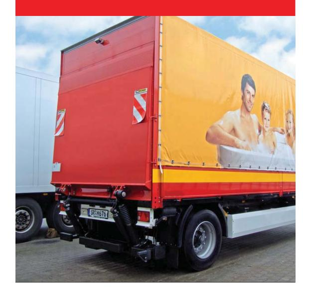
1500 / 2000 KS tail lifts benefit from the well-proven standard components of 1500 / 2000 K lifts. The lift has been specifically designed for vehicles with very little overhang on the rear of the vehicle. The lift mechanism is available with 4 different lift arms.
