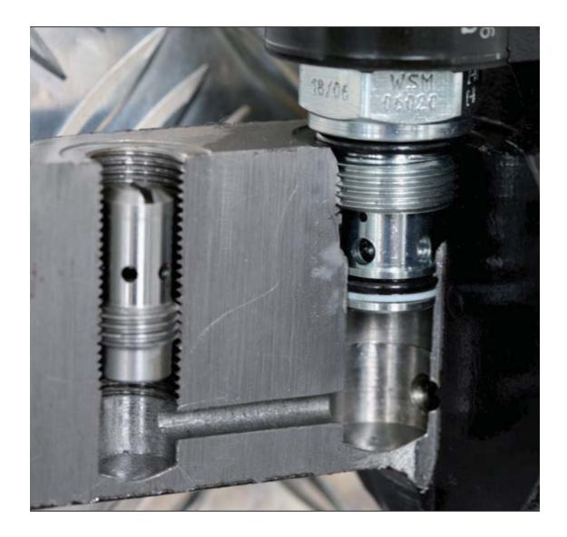
Every cylinder is fitted with flow control valves which safely control the descent of a fully loaded platform, even in the event of a burst hose in the hydraulic circuit.
