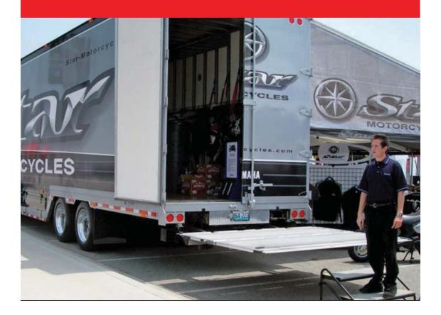
Heavy duty retractable lift available in two capacities. Stowing 'completely' out of the way under the rear of the vehicle it is ideal for fork lift and dock loading operations. Suitable for dry freight and refrigerated applications.
