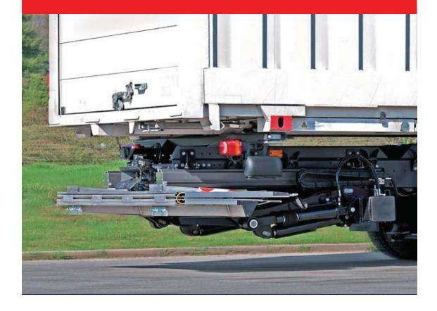
The 2000 KLUZ is a robust lightweight retractable lift. A push-pull cylinder aligned lengthwise moves the lift into the desired position. The lift leaves the factory fully assembled and with the lift unit KTL coated, ready for clamping onto the chassis supplied with kits suitable for trucks or trailers.
