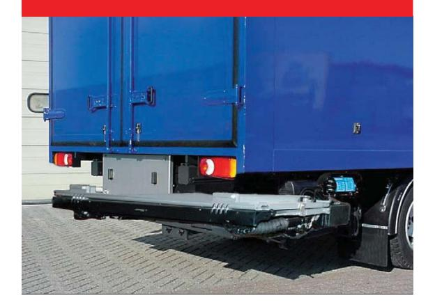
Robust retractable lift available in two capacities with double folding platform ideal for vehicles with short overhangs (from 985 mm). Stowing 'completely' out of the way under the rear of the vehicle it is ideal for fork lift and dock loading operations. Suitable for dry freight and refrigerated applications.
