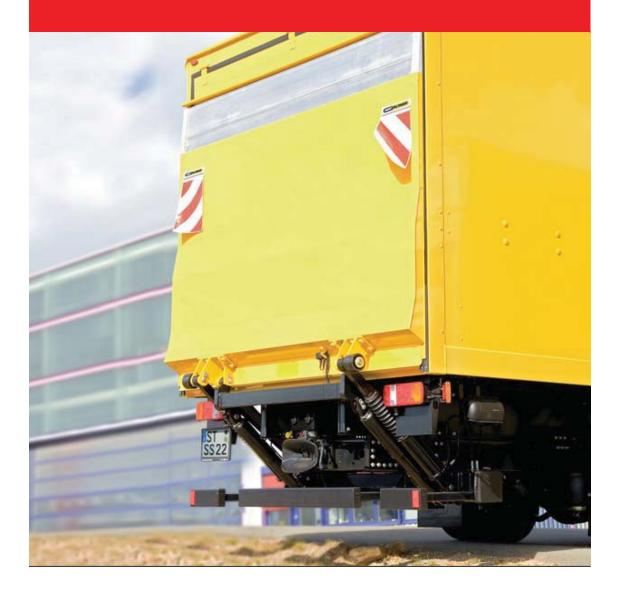
Probably the most reliable, heavy duty lift on the market with a lifting centre of 1000 mm. Suitable for a wide range of applications and fits most vehicle bodies and trailers. The 4-cylinder lift mechanism is available with 5 different lift arms, ranging from 700 mm to 1100 mm. Both steel and aluminium platforms are 'made to measure' available up to a maximum depth of 2800 mm.
