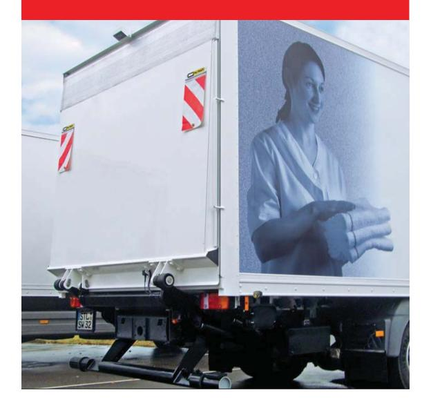
Special applications require special equipment. With its exceptionally large load clearance of 1000 mm and its lifting capacity of 2500 kg, the 2500 KK is rightly considered one of the most powerful tail lifts in its class. It is designed for a wide range of applications such as food and beverage distribution, and for drawbar units.
