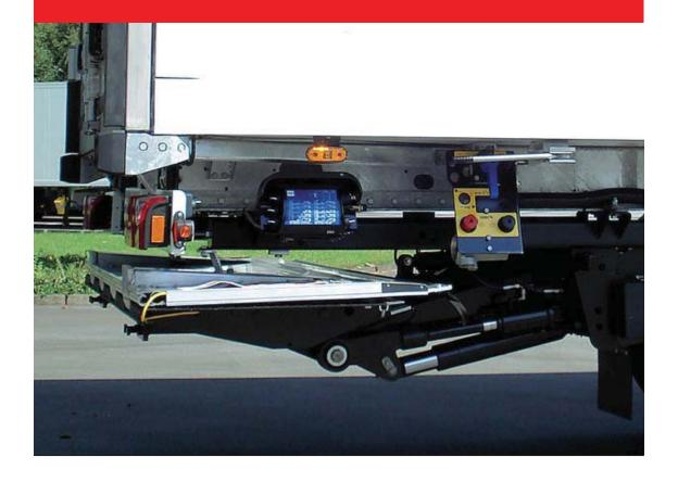
A specially designed retractable tail lift for easy assembly on semitrailers with a frame width of approximately 1300 mm.
